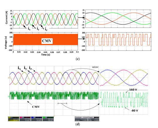
**Figure 6.** Each phase current and CMV for Case 2, first considering *PPPP* as the switching state: (**a**) Simulation result, (**b**) Experimental result; and considering *NNNN* as the switching state (**c**) Simulation result, (**d**) Experimental result (I = 10 A/div., CMV = 200 V/div. and 10 ms/div.).
