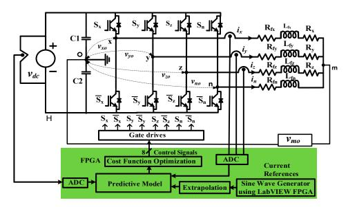
Figure 1. Three-phase four-leg inverter with a field programmable gate array (FPGA) control block.
