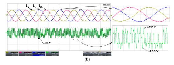
**Figure 5.** Each phase current and common mode voltage (CMV) for Case 1 (**a**) Simulation result, (**b**) Experimental result (*I* = 10 A/div. CMV = 200 V/div. and 10 ms/div.).
