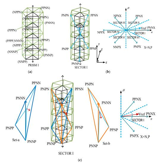
**Figure 2.** (a) Switching vectors and prisms (b) Projection of a sector on the  $\alpha\beta$  coordinate (c) Sector identification with near state vector selection (NSV).
