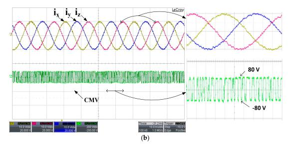
**Figure 7.** Each phase current and CMV for Case 3 (a) Simulation result, (b) Experimental result (I = 10 A/div., CMV = 200 V/div. and 10 ms/div.).
