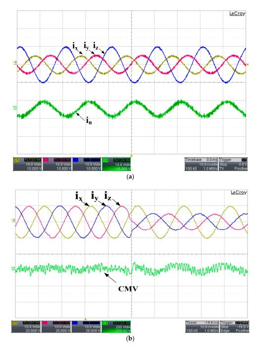
**Figure 9.** (a) Unbalanced references in phase -*y* and -*z* from 10 A to 5A with balanced resistive loads and filters, and (b) Step change in phase -*y* and -*z* references from 10 A to 5A with the proposed NSV-MPC technique.
