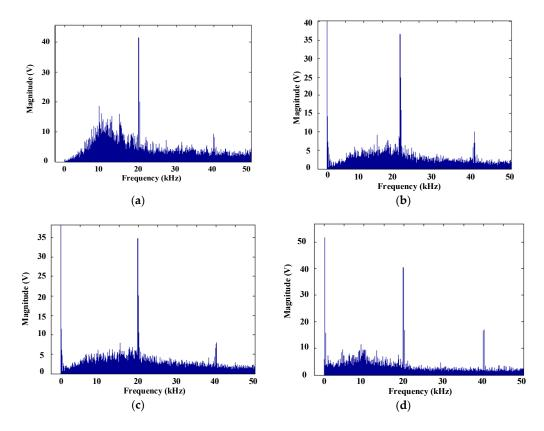
**Figure 8.** FFT analysis results of CMV (**a**) Conventional MPC, (**b**) Proposed NSV-MPC with *PPPP* vector, (**c**) Proposed NSV-MPC with *NNNN* vector, (**d**) Proposed NSV-MPC with active vectors only.
