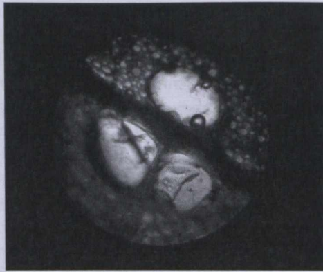
Figure 5: Microscopic image and 400X of transversal sections of samples treated with animal glue and Mowilith 20. Fibers and vessels lumina approximately appeared filled with consolidant.
