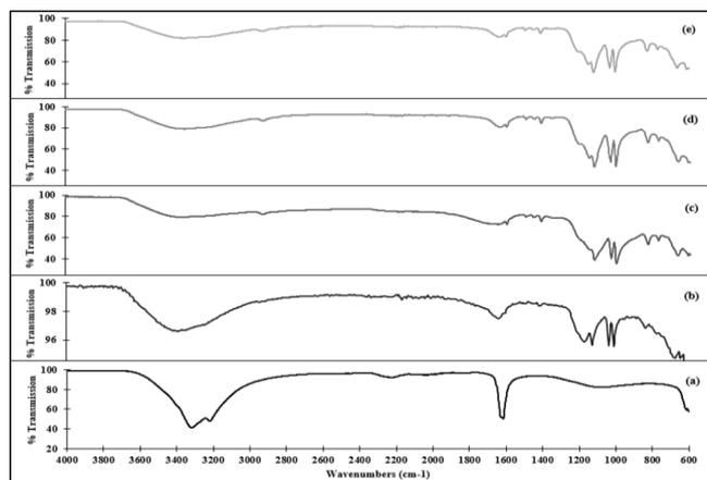
Figure 1. (a)  $\text{SmCl}_3 \cdot 6\text{H}_2\text{O}$  salt. (b) Fresh Amberlite IR-120  $\text{H}^+$  beads. (c) Amberlite IR-120  $\text{H}^+$  ground and sieved to size 20 – 40  $\mu\text{m}$ . (d) Amberlite microparticles labelled with  $\text{SmCl}_3 \cdot 6\text{H}_2\text{O}$  salt. (e)  $^{153}\text{Sm}$ -Amberlite microparticles after 6 h neutron activation.
