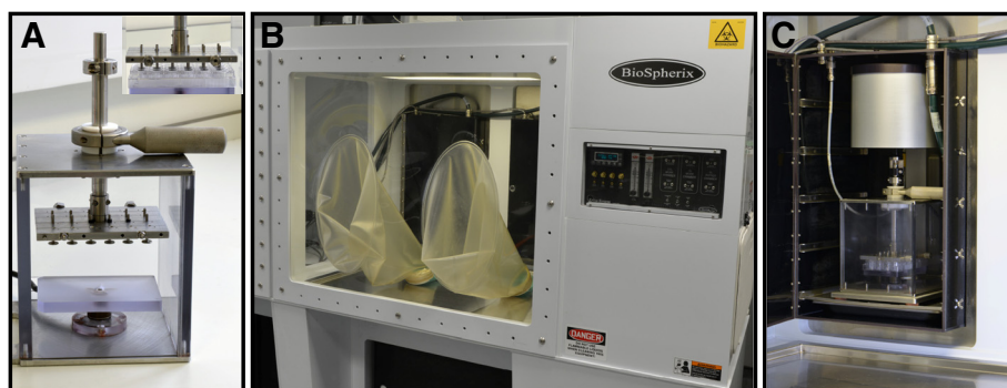
Figure 1 The ex vivo system. Bose bioreactor (A) integrated with the Biospherix (B) to facilitate uninterrupted ex vivo conditions, under controlled oxygen tension within the incubator (C). The inset in (A) shows custom designed compressive mounting plate with loading pins positioned above a 24-well culture plate.
