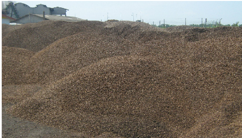
Figure 1. The great mass of oil palm shells (OPS) in the palm oil mill area.
