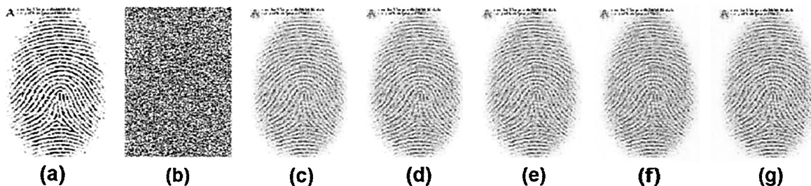
Fig. 2. (a), Original image; (b), original image (a) with 80% salt-and-pepper noise; and (c)–(g), image restored from memory of 10 different simultaneously stored fingerprints after presentation of the “query-image,” which is (c) whole original image (a), (d) 25%-occluded image (a), (e) 50%-occluded (a), (f) 75%-occluded (a), and (g) noisy image (b).
