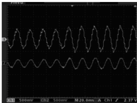
Fig.12. The load phase voltage v_{aN} and the line current i_a (150V/div, 5Amp/div, 20ms/div).
