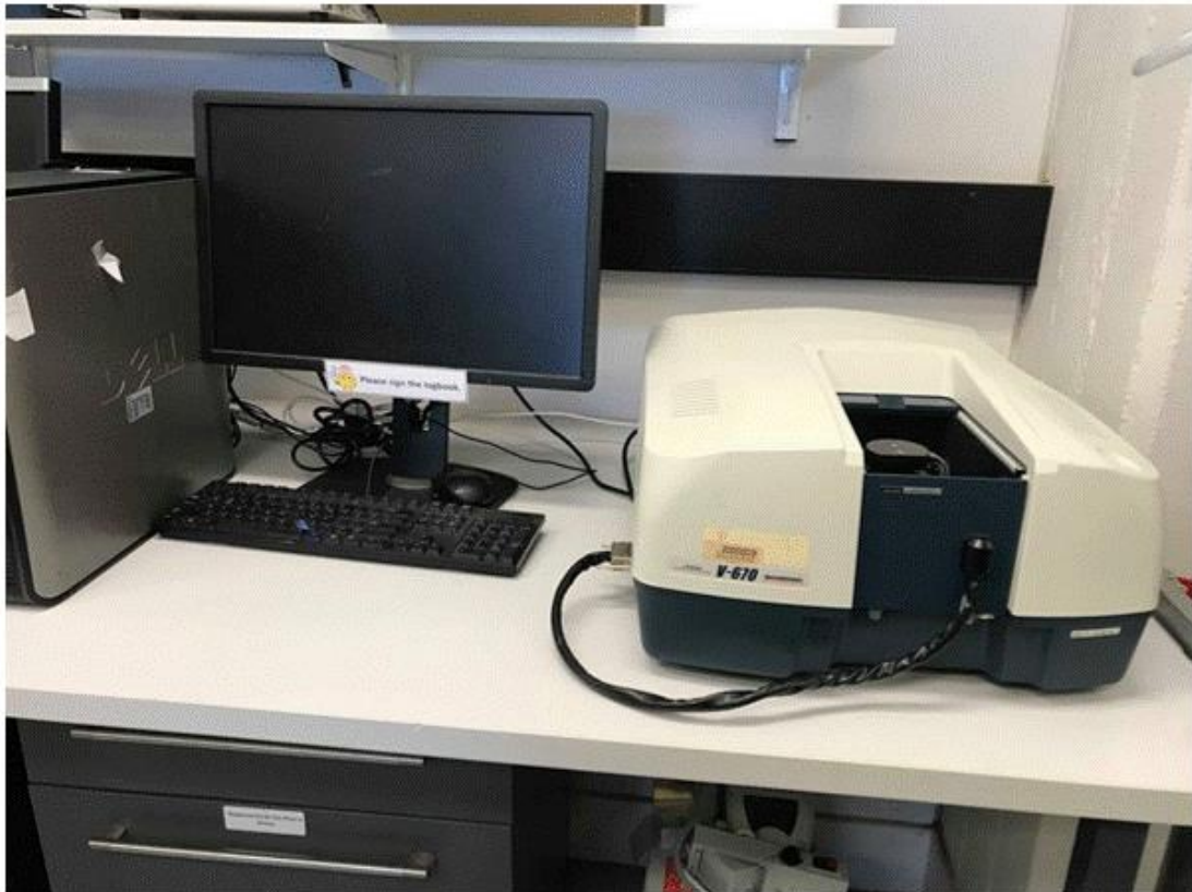
Figure 3.6: UV-670 JASCO, USA double beam spectrophotometer.
