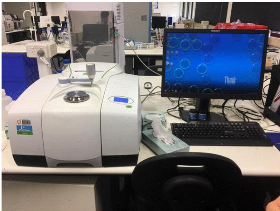
Figure 3.5: PerkinElmer Spectrum 100 FTIR Spectrometer, USA.
