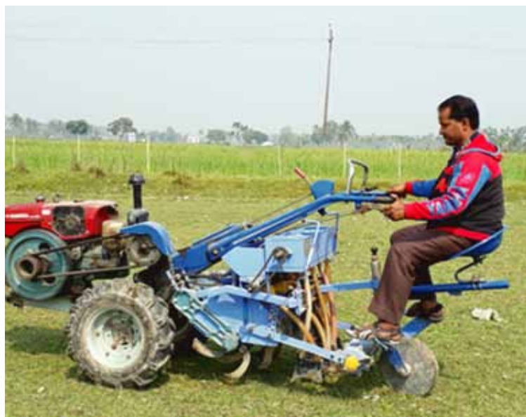
Figure 6: The VMP attached to 2-wheel tractor in operation.
