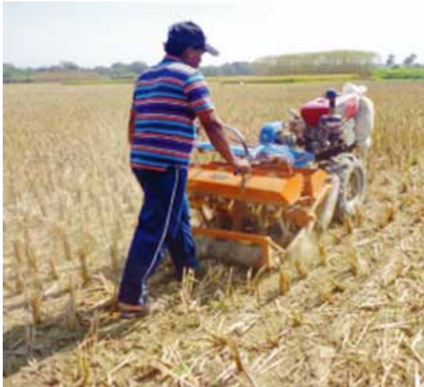
Figure12: Optimum stubble height/level suitable to operate planter.
