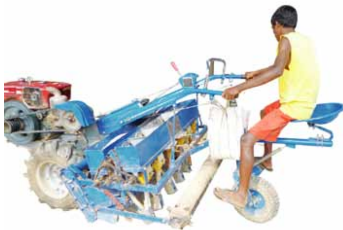
Figure 9: The Versatile Strip Seed Drill (VSSD) developed in Bangladesh under the funding support of ACIAR.
