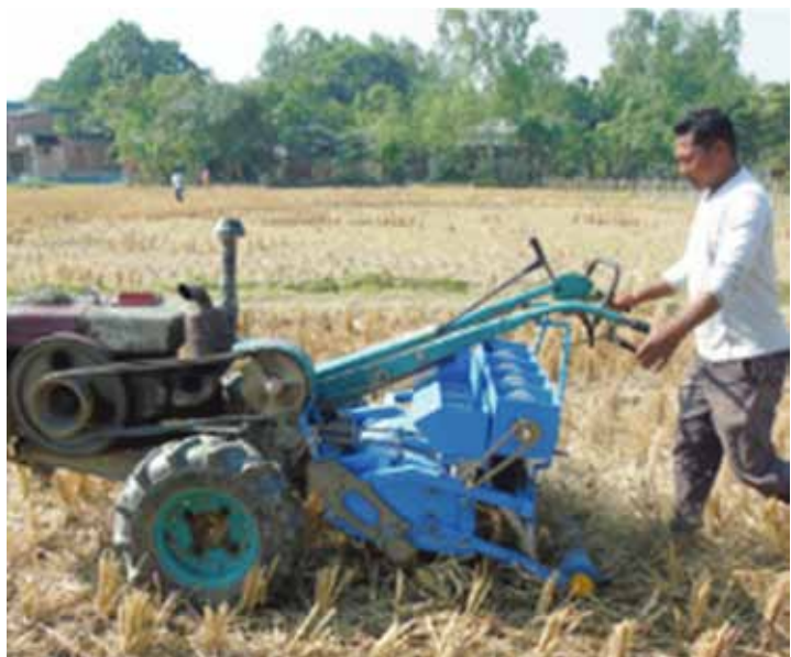
Figure 2: Alluvial soil, having 20-30% of moisture and 20 cm height of rice stubble is most preferable land type to operate the 2WT-based planter.
