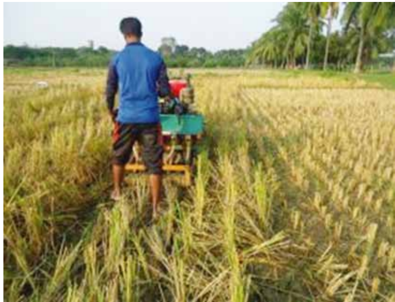
Figure 4. A Versatile Multi-crop Planter in use for strip planting.
