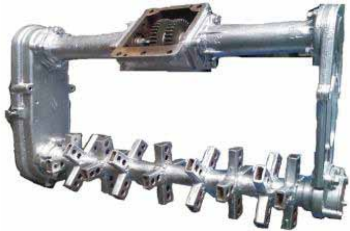
Figure 7: Re-designed rotary shaft of VMP that is suitable to sow varied row spacing of crops in different tillage mode.
