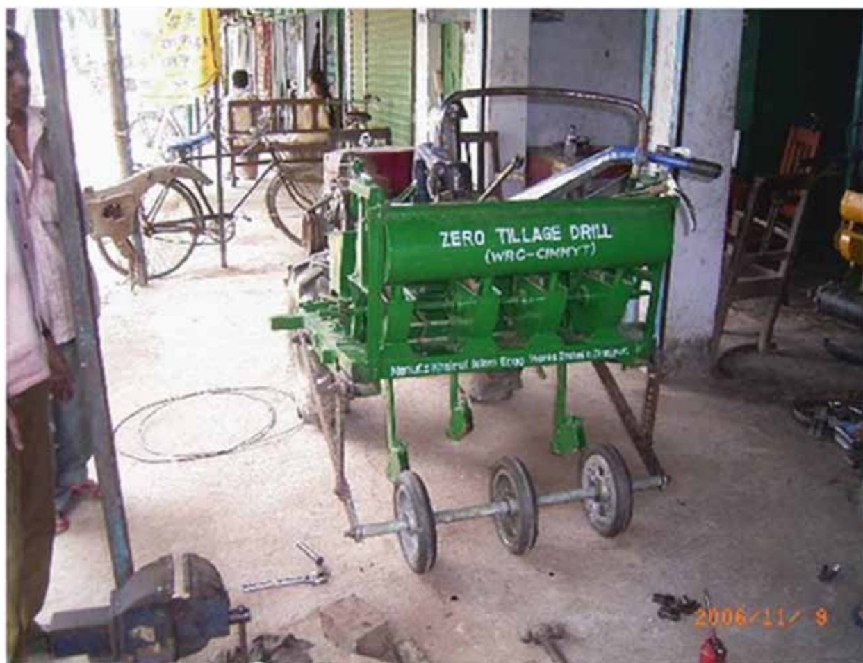
Figure 5: The toolbar mounted Zero Tillage Planter developed in Bangladesh with the funding support of ACIAR.
