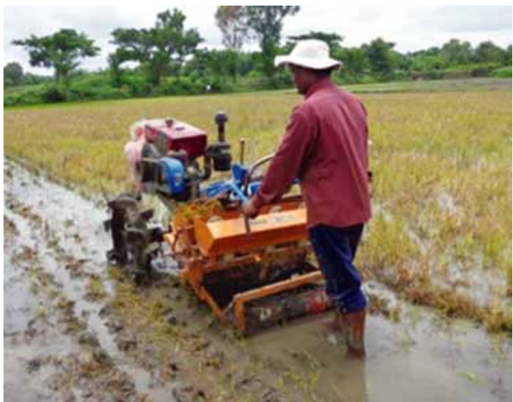
Figure 3: VMP operating in wet field to show seed. This should be avoided.
