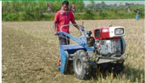
Figure 11: The PTOS pulverizes soils more than conventional tillage.
