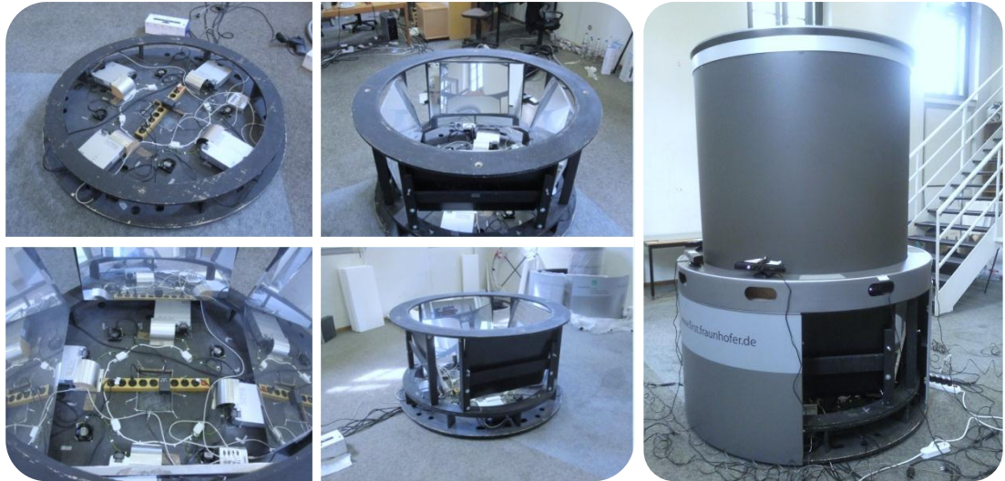
Figure 5.3: Column base with beamers and deflection mirrors and integration of sensor covers.
