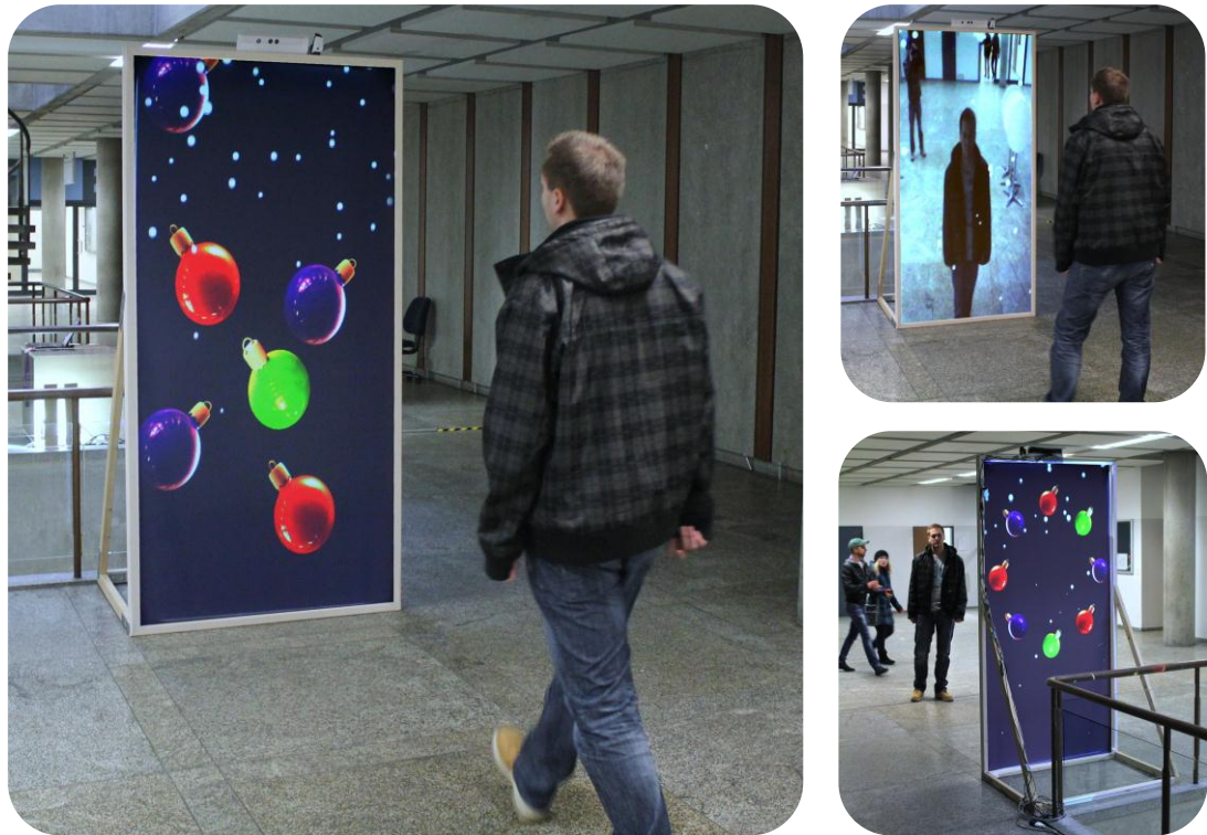
Figure 5.5: Lightweight Interactive Life-size Display that can display one person in life size.
