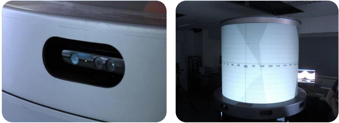
Figure 5.4: Unobtrusive integration of Kinect sensors and fine calibration of the cylindrical image.
