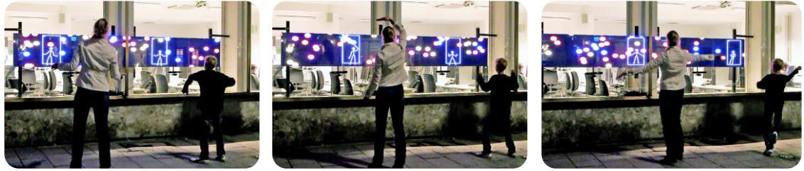
Figure 10.6: Users being subtly directed along the display by imperceptibly moving visual cues.
