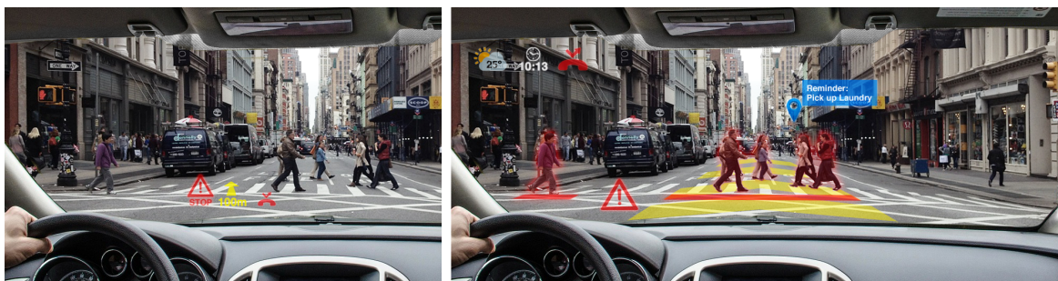
Figure 1.1: The left image shows an exemplary head-up display of conventional size. It indicates the limited display space and content capacity. The right image visualizes a futuristic 3D windshield display. This mockup uses the entire windshield as display space and presents additional content to the driver.
