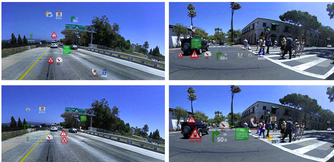
Figure 4.3: The upper left image shows how the applied view management (first version) could look like when content is displayed in every information space. The remaining three images show example layouts created by the drivers who participated in the AV simulation study. The images show 2D versions of the driving scenes in which the drivers had to place content.
