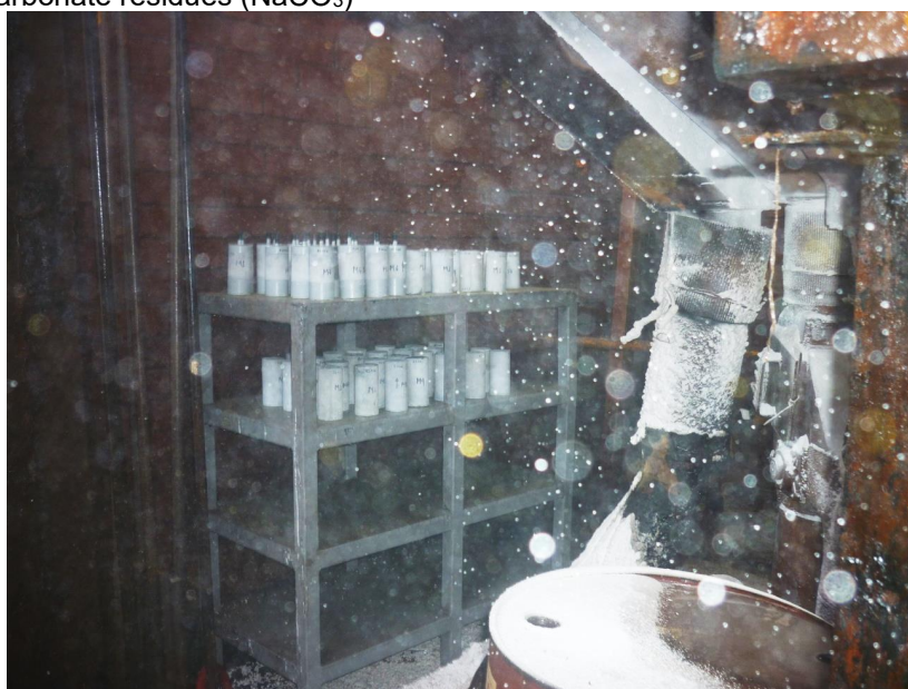
Fig. 1 - Appearance of the surroundings of the production plant (precipitating \text{CaCl}_2 ).
