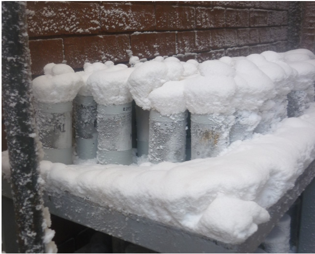
Fig. 4 - Specimens exposed to industrial environment.
