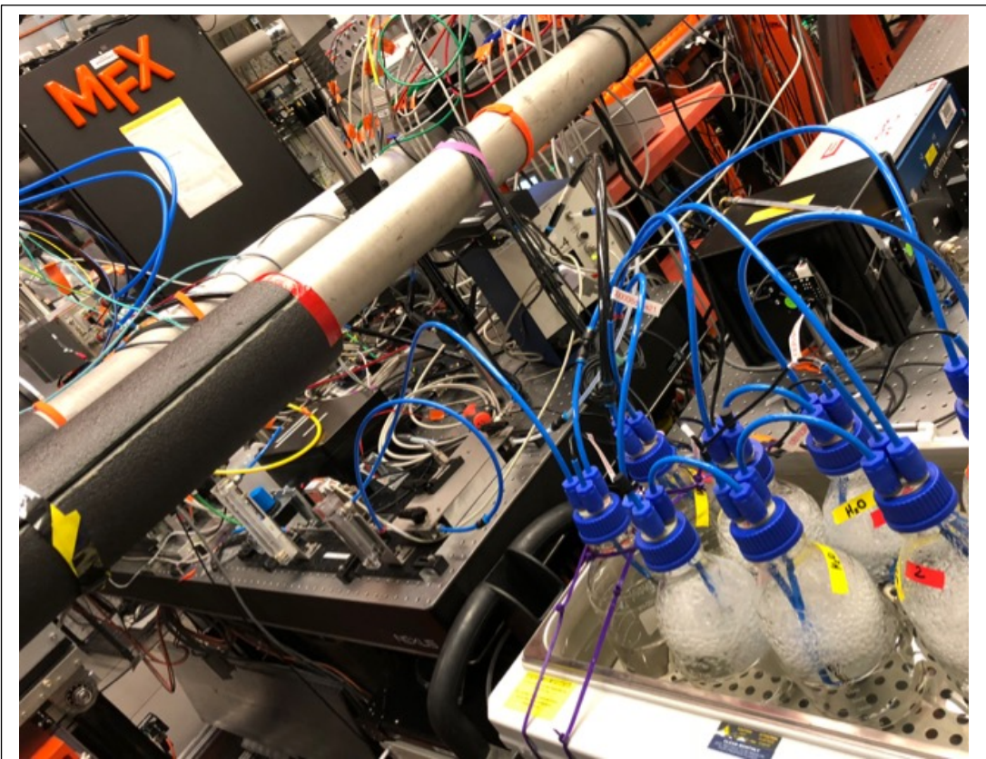
Figure 3.18: Humidity set-up to maintain crystal hydration.
