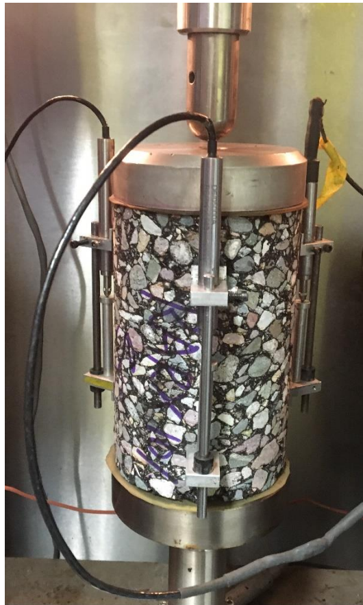
Figure 22. Instrumented Dynamic Modulus |E^*| Test Sample
