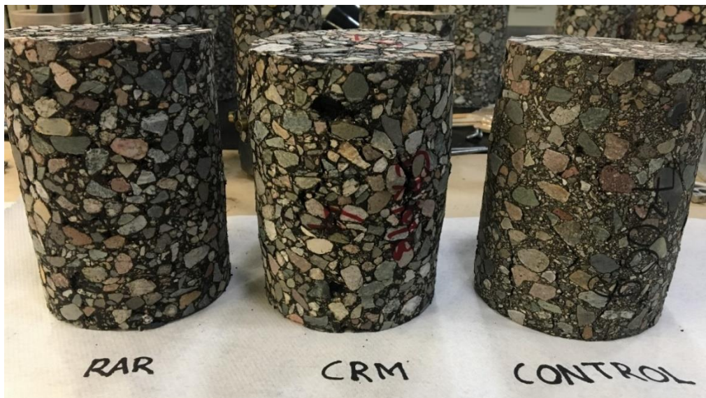
Figure 35. Deformed Samples After Flow Number Test
