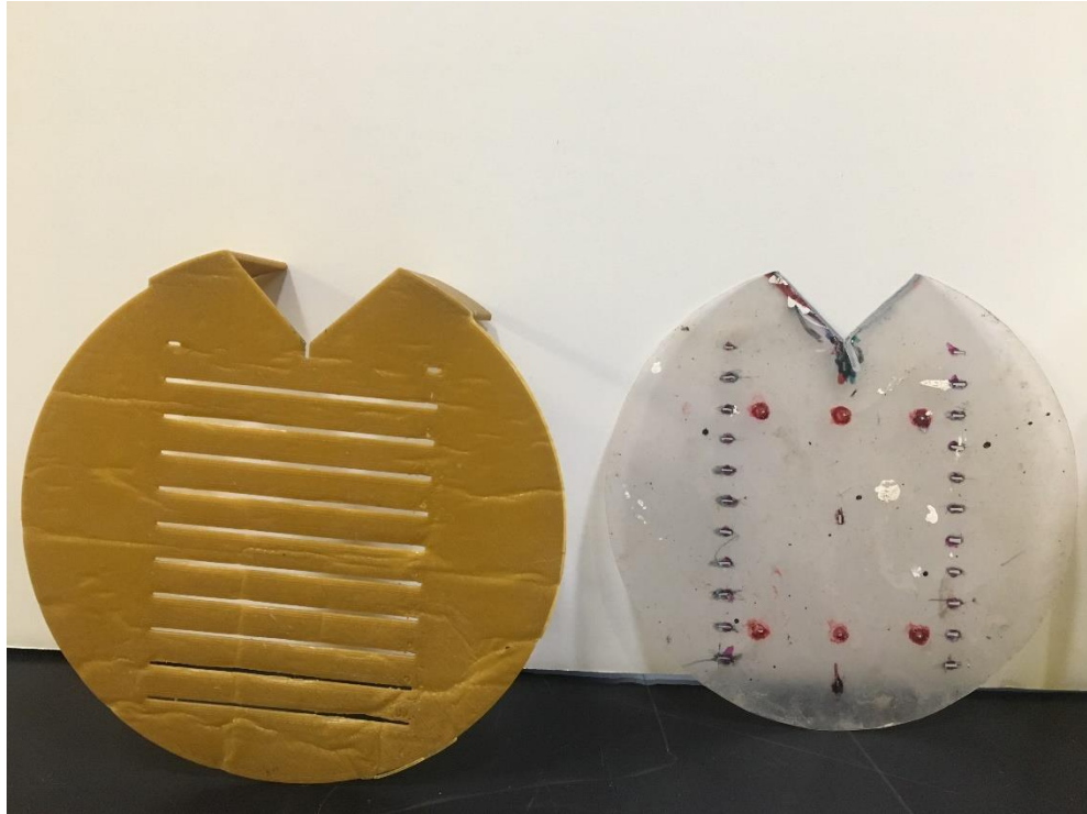
Figure 26. 3D Printed Template Used for C* Fracture Test Sample Markings
