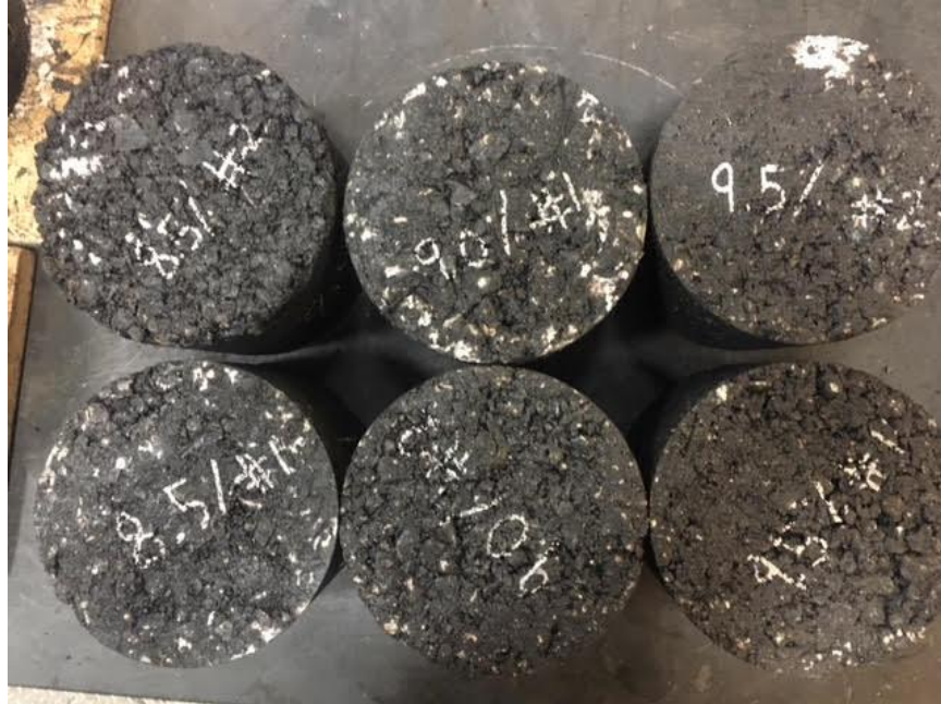
Figure 18. Compacted Superpave Mix Design Samples for RAR Mixtures
