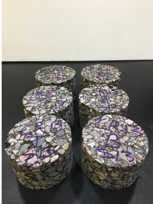
Figure 24. Dry and Wet Conditioning Subsets for TSR
