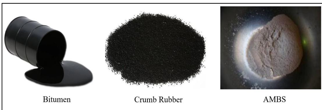
Figure 10. Composition of RARX (Source: Consulpav 2013)
