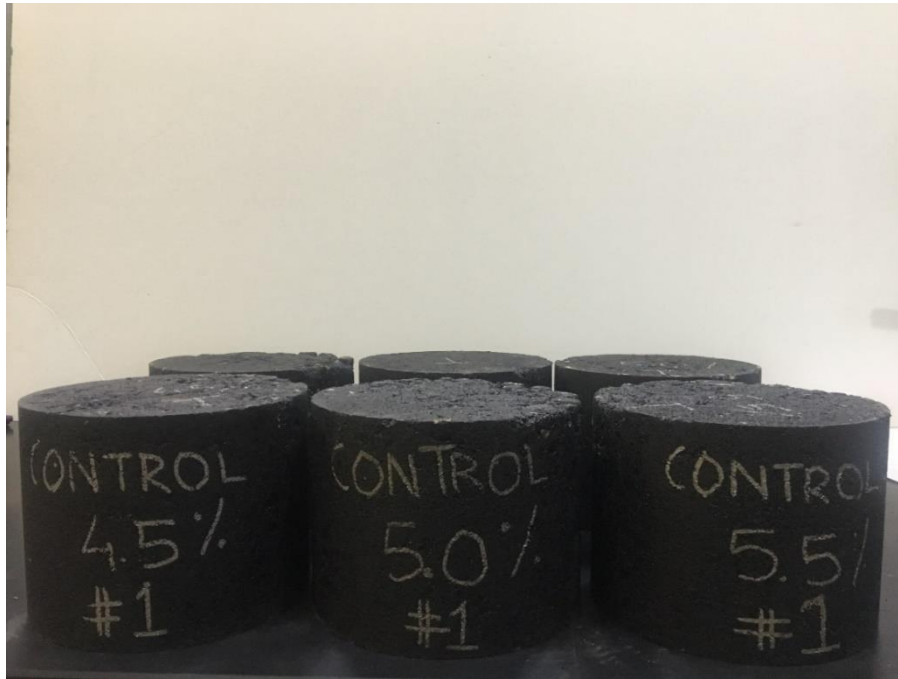
Figure 20 Compacted Superpave Mix Design Samples for Control Mixtures
