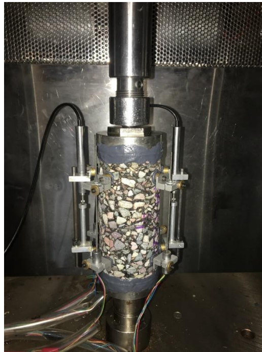
Figure 27. Mounted Axial Cyclic Fatigue Sample
