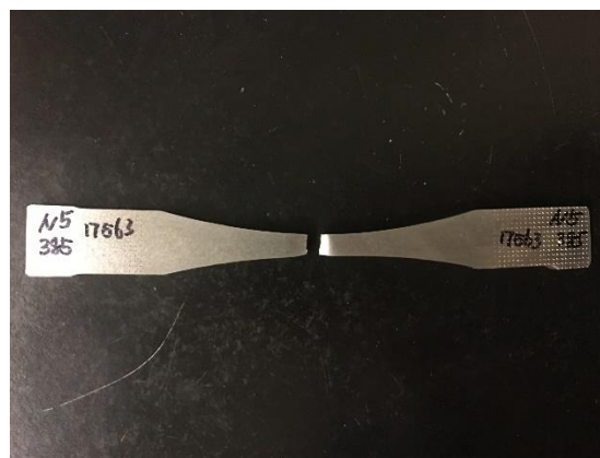
Figure 10 Fractured fatigue specimen.
