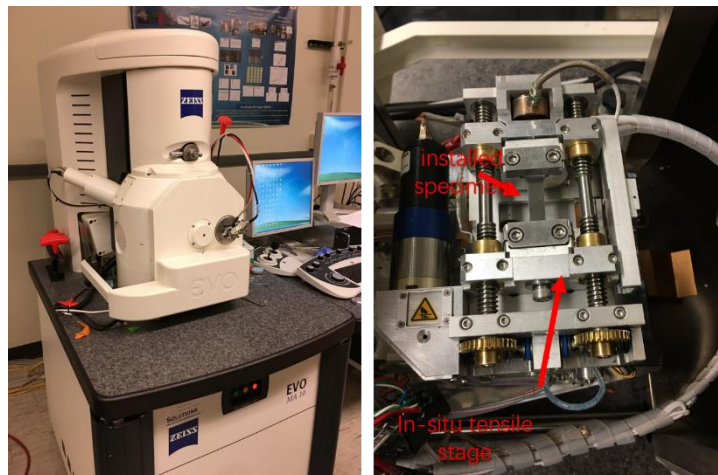
Figure 21 (a) ZEISS EVO MA 10 SEM; (b) in-situ SEM fatigue testing setup.
