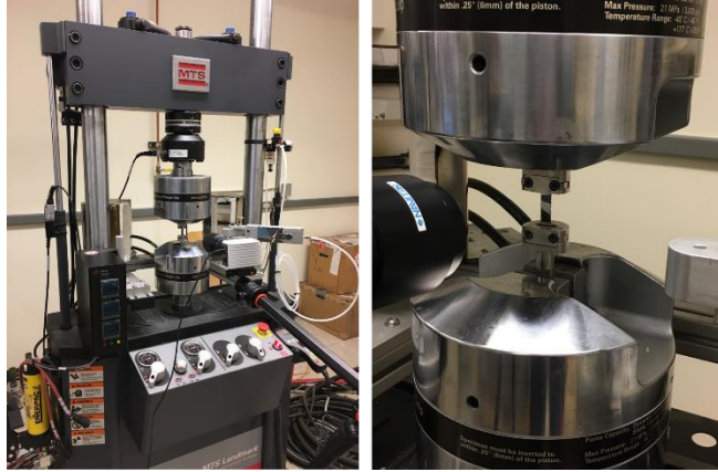
Figure 19 Specimen precracking setup.
