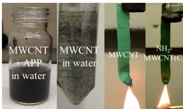
Figure 4.10 Images of MWCNTs dispersed with and without APP in water and the flame retardancy test on the sample spray coated on polyester fabric with reference image of \text{NH}_2\text{-MWCNT(C)} coating as classification I.
