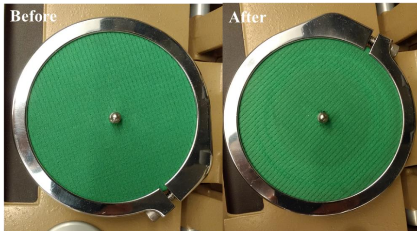
Figure 5.6 Pictures of MWCNT-APP coated polyester fabrics before (left) and after (right) the mechanical abrasion.
