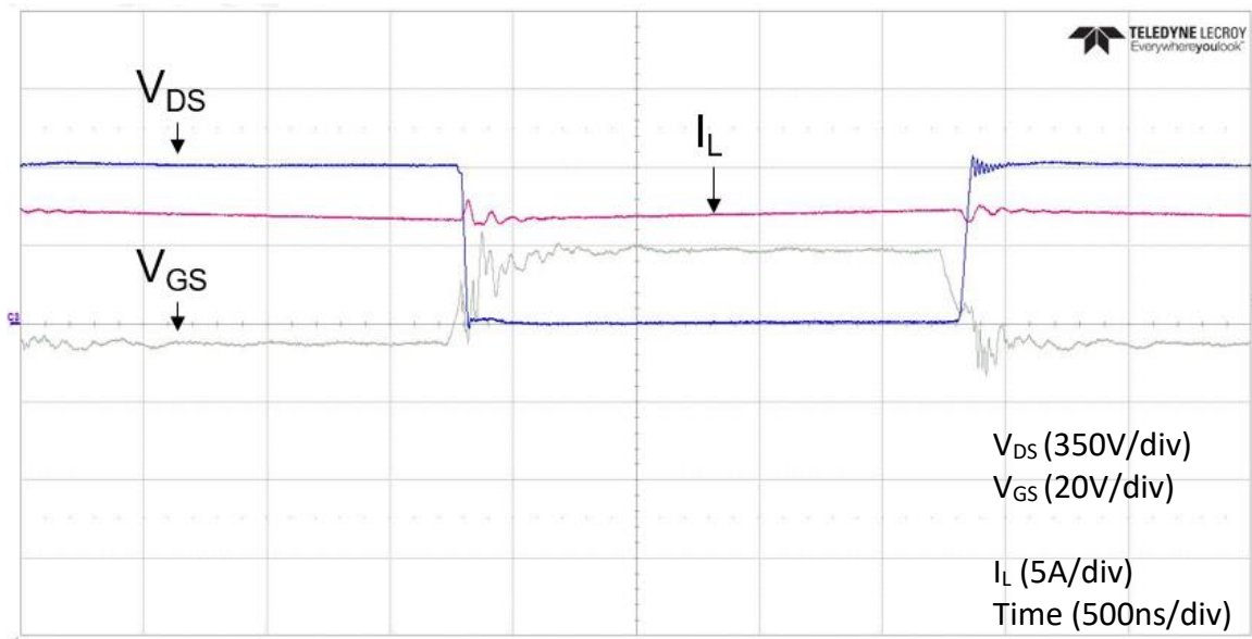
Figure 4.4: Hard-switched test waveforms for 1.35kW power rating
