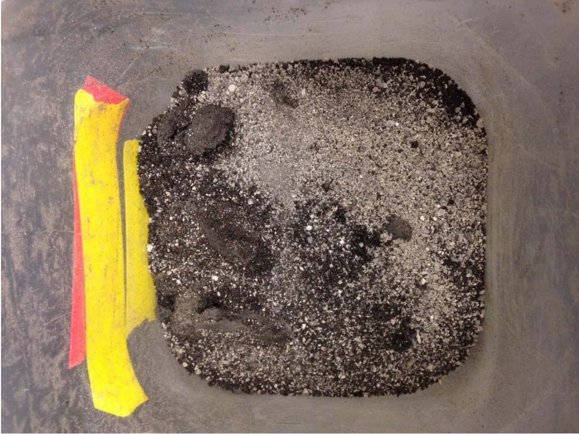
Figure 4.5. BM3 soil after smoldering. The soil took on a white color.
