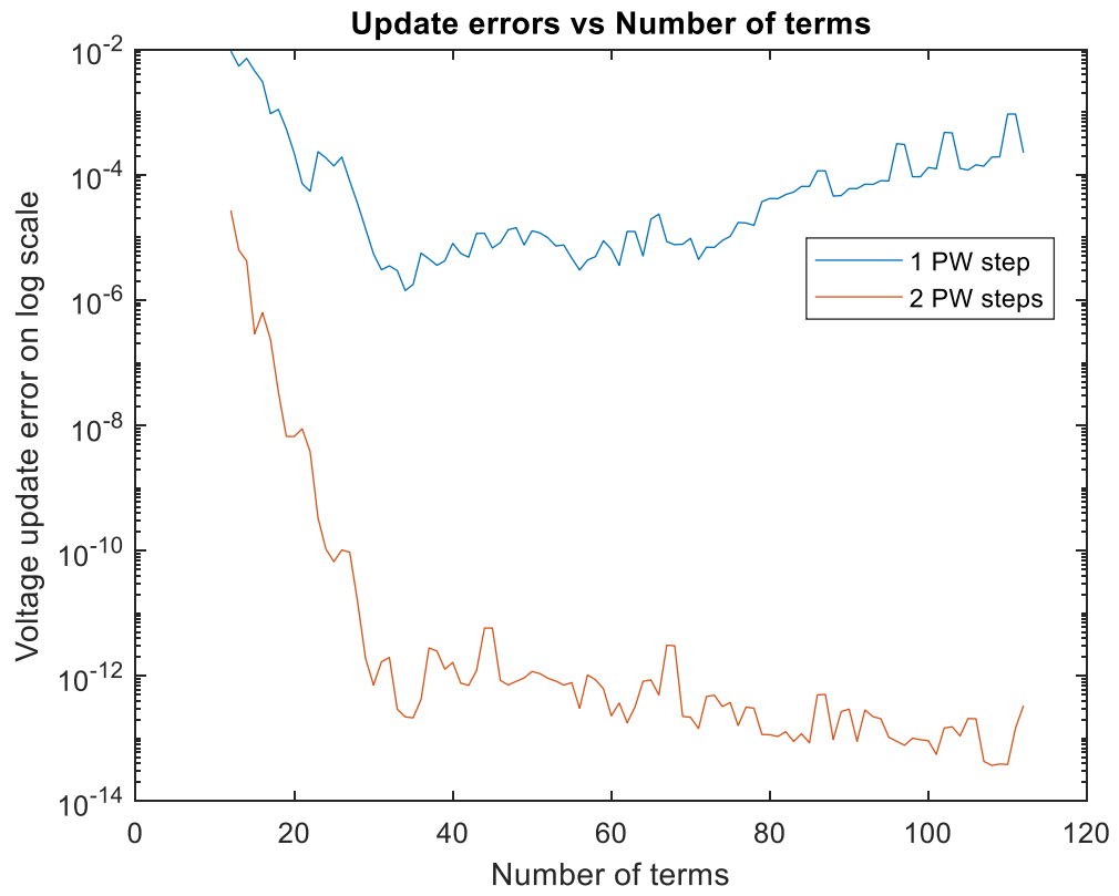
Figure 4.13 Voltage update error vs. number of terms in series using P-W method
