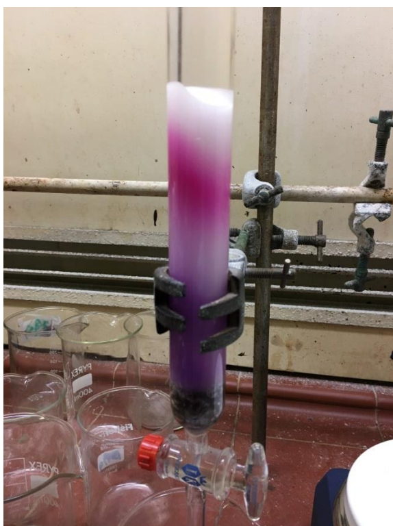
Figure S7 The separation of the mauveine (purple) and N-tert -butylmauveine (red) bands.
