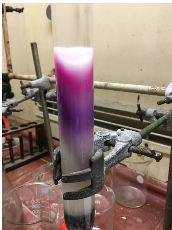
Figure S6 The separation of the mauveine (purple) and N-tert -butylmauveine (red) bands.
