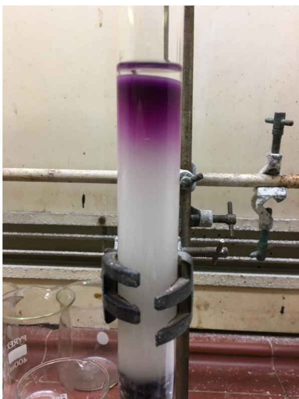
Figure S5 The crude mauveine band at the start of the column.
