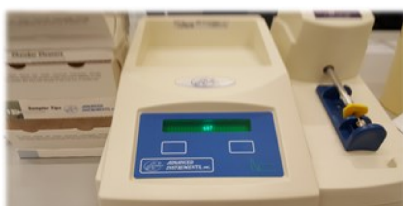
Figure 2. Freezing point osmometer. We have two of these stationed around the lab so that students can accurately measure osmolality. The osmometers may also be staffed by a demonstrator or member of technical staff who can talk to small groups of students about the importance of accuracy and calibration. If a lab has no access to an osmometer, values can be provided for the students and they can still work out which sample came from which person.
