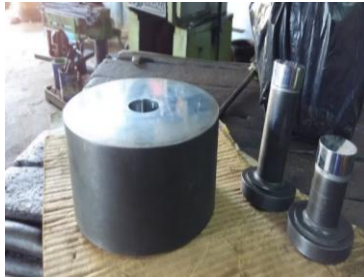
Fig 3.1 Die and Punch for Compaction
