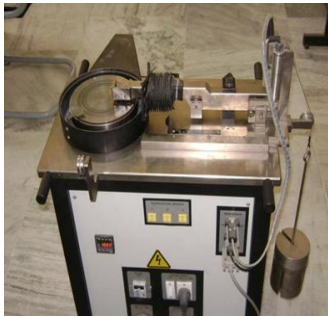
Fig 4.1 Pin-on-Disc Tribometer Setup Fig 4.2: Wear Test Specimens
