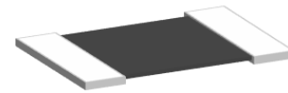
Figure 1. A Schematic of a Nanocomposite Sample Prepared for Electrical Conductivity Measurement by Two-Wire Technique
