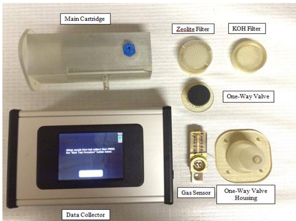
Fig. 1 - Layout of the breathalyzer including each component
