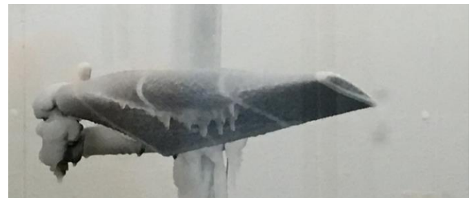
Figure 5. Ice accretion on a wind turbine blade at V = 5\text{ m/s} and \alpha = 45^{\circ} after 3 hours of icing conditions.
