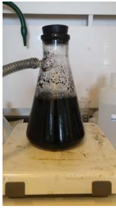
Figure 2. PDMS/CNT Solution - Chloroform Expulsion
