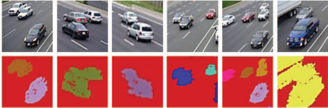
Figure 4.1: Example vehicle clusters formed in dense traffic conditions (Top row), and corresponding results from a 2D segmentation algorithm (Bottom row).
