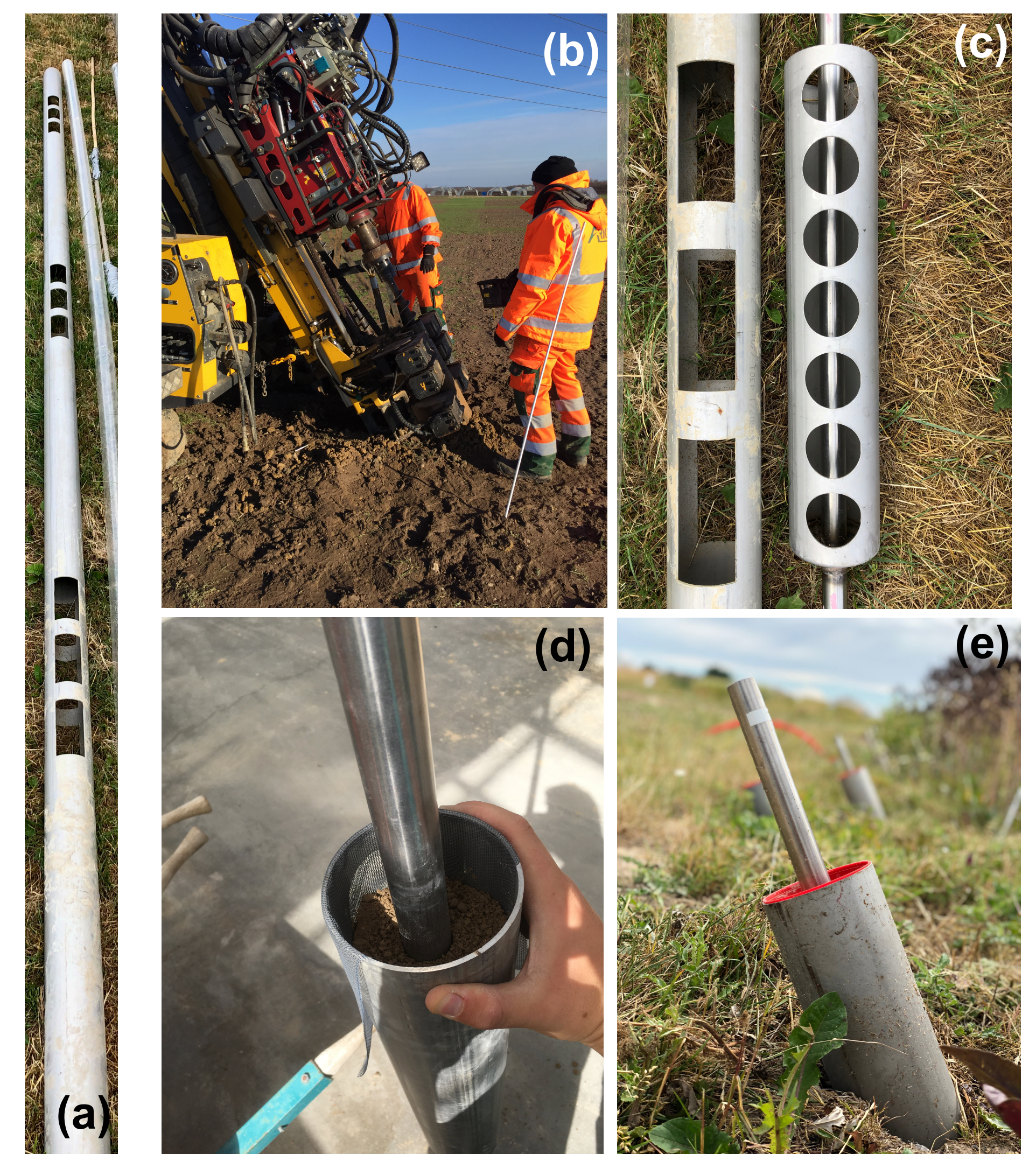
Figure 2: A 5.85 m-long access-tube with 3 openings (a); Drilling of an access-tube (b); A matching-view of ingrowth-core and access-tubes opening (c); Re-packing of labelled soil into the ingrowth-core (d); Ingrowth-core placed into the access-tube in the field (e).
