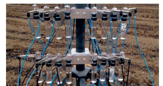
Fig.3 Quantification of NH 3 -emissions via automatized "Low cost impinger system (LOCI)". [5]
