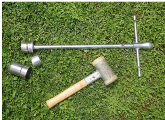
Figure 2. Hammer-driven double-cylinder sampler
