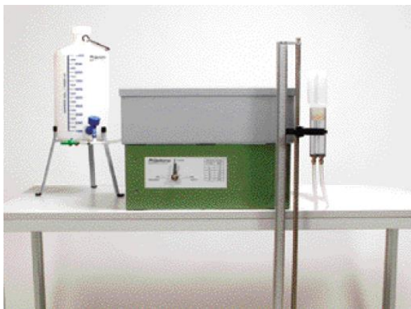
Figure 3. Sand box (left) and pressure plate extractor (right)
