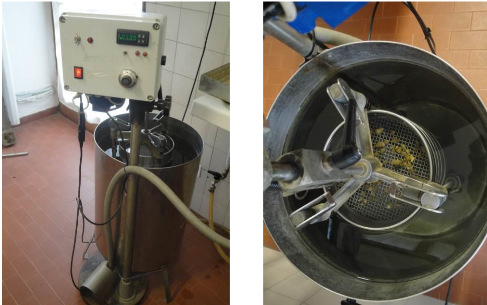
Figure 7. The electronic-controlled machine for aggregate stability analysis by wet sieving.
