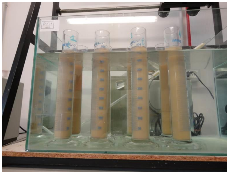
Figure 5. Soil particle-size analysis by the pipette method.
