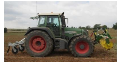
Terminated ASC cover with roller crimper
