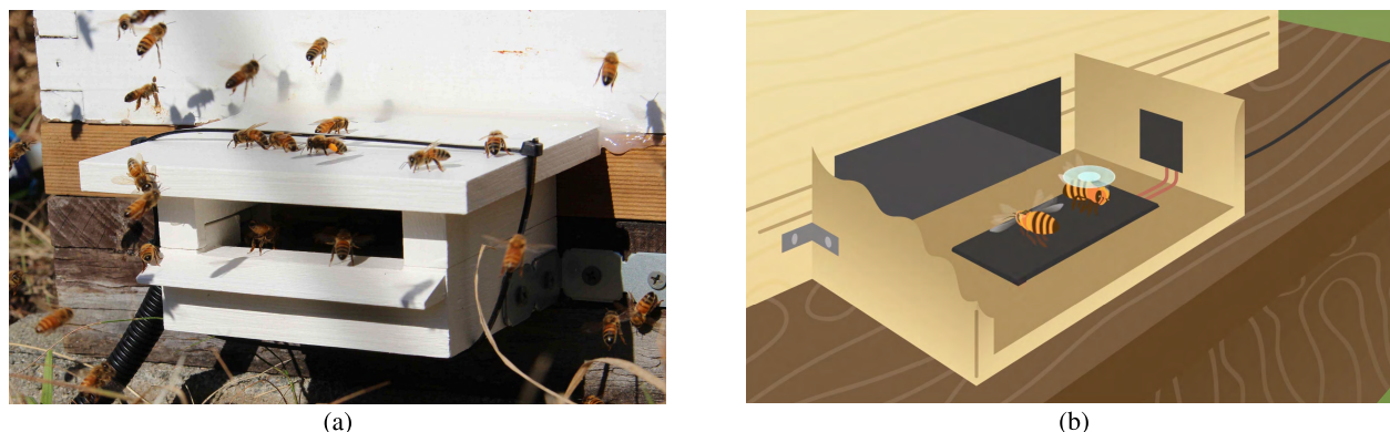
FIGURE 1. The bee experiment conducted at Geeveston, Tasmania: (a) hive entrance; and (b) RFID reader installed underneath the entrance that detects the passage of tagged bees.
