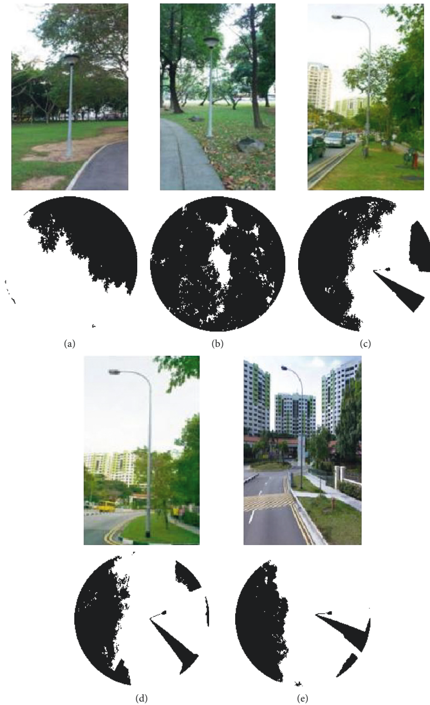
FIGURE 2: Photos and fisheye photos for each location (measurements were taken at 2.0 m above the ground level). (a) Point 1 (SVF = 0.61). (b) Point 2 (SVF = 0.17). (c) Point 3 (SVF = 0.48). (d) Point 4 (SVF = 0.66). (e) Point 5 (SVF = 0.67).
