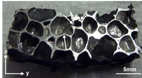
Fig. 47 Cross-section of a foam specimen after 5 laser scans at 180 W and 10 mm/s. The laser was scanned into the page. The white arrows show where cell walls were bent during laser forming, indicating that the foam cannot withstand high compressive stresses.
