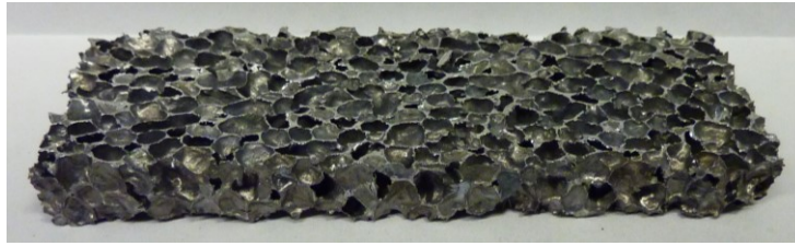
Figure 7: Metal foam that was used in chapters 2 & 3.
