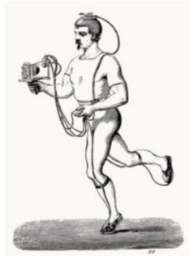
Figure 26: Sphygmograph and Step-Tracker developed by Etienne Jules Marey in 1860.
