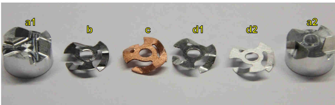
Figure 6.6: Home designed mold and molded brackets of different materials. a1,a2: the male and female mold respectively; b: 0.05 mm Ta film bracket; c: 0.4 mm Cu sheet bracket; d1,d2: 0.2 mm Al sheet bracket.
