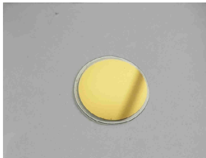
Figure 6.4: A 200 nm Au coated \text{Ø}10 mm, 0.1 mm thick \text{LiTaO}_3 single crystal. \sim 20 nm Cr is first deposited as the intermediate layer for the adhesion of Au layer. The \text{LiTaO}_3 single crystal was obtained from SurfaceNet GmbH.
