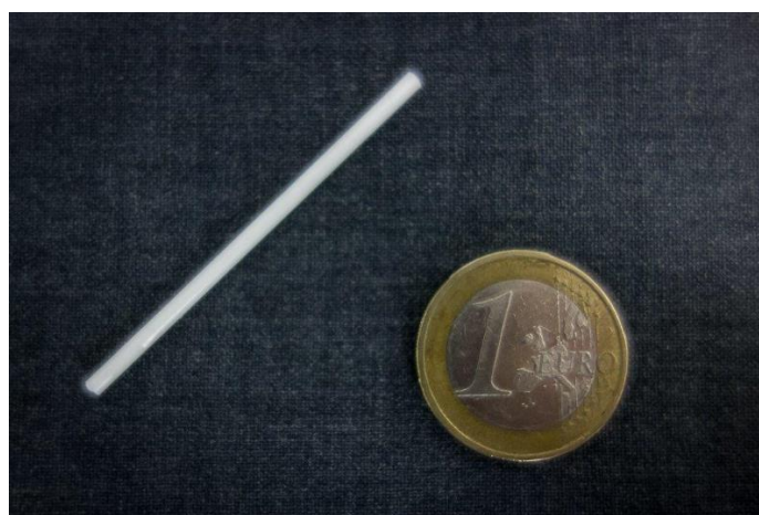
Figure 4.1. The analysed column packing (Acquity UPLC BEH C18 1.7 \mu\text{m} , 2.1 \times 50 mm) after its embedding in poly(divinylbenzene) and the subsequent extrusion from the encasing 2.1 mm inner diameter, 50 mm long stainless-steel column.
