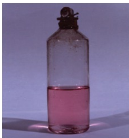
Figure 4. Colloidal gold NPs by Michael Faraday, which are reproduced by courtesy of the Royal Institution of Great Britain [43] .
