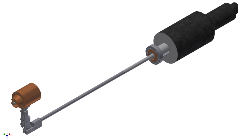
Figure 2.8: Assembled Heater for Crystal Samples — Assembled heater for crystal samples as designed by O. LYTKEN with a linear/rotational motion feedthrough a and a light bulb b filament for sample heating.
