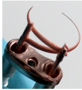
Figure 6.27: Copper Glazed Filament — The filament a on its mounting posts after evaporation of approximately 4 g of copper from a molybdenum crucible b in the electron beam evaporator c . Although the filament is incomplete in this picture, it is clearly visible that the thickness of the copper deposit decreases from the mounting posts to the center of the filament, which is the hottest zone during operation.
