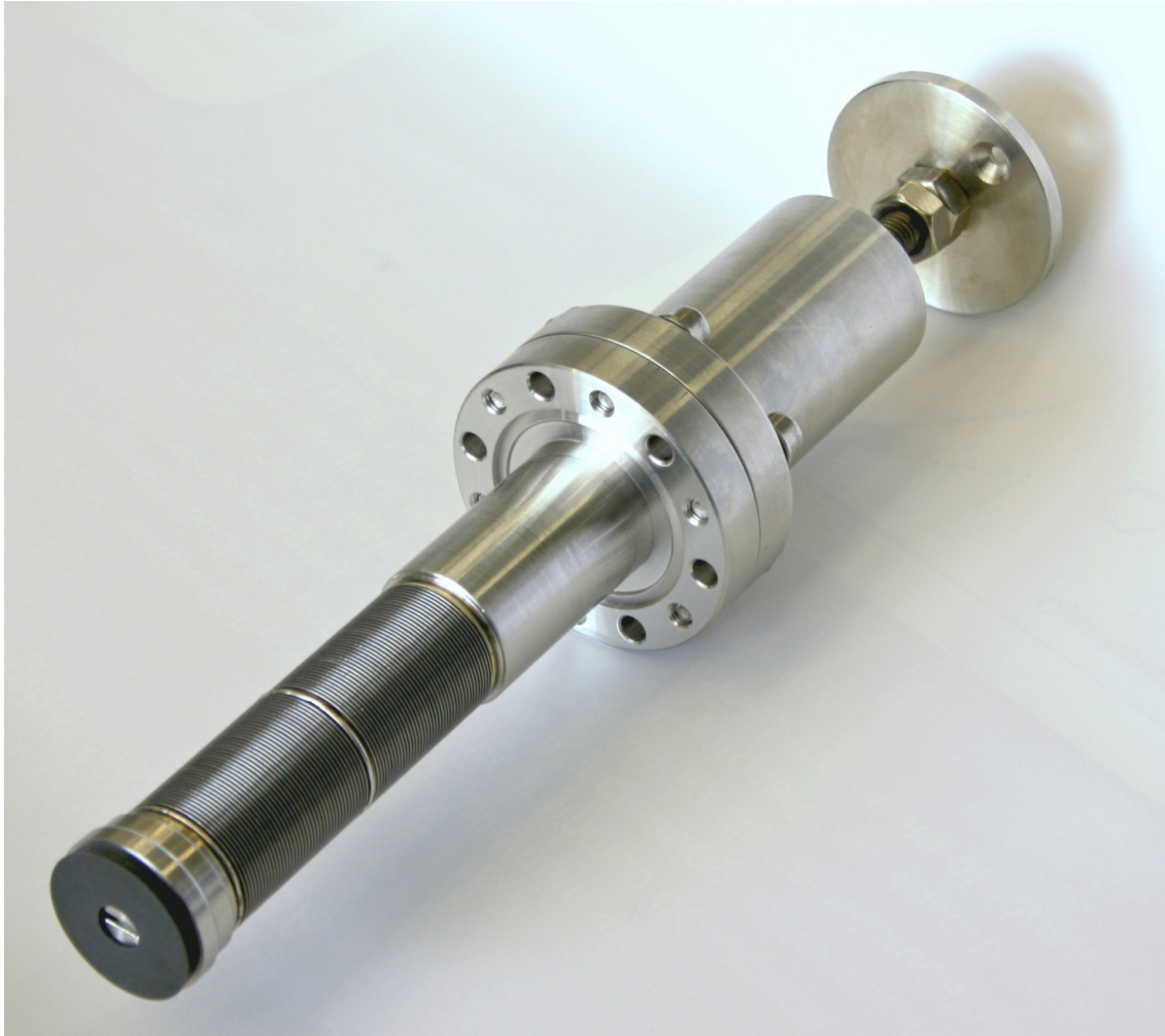
Figure 2.25: Assembled Valve — A photograph of the preliminary assembly of the valve as described in Figure 2.24 is shown. The mount of the flat gasket has been altered later.
