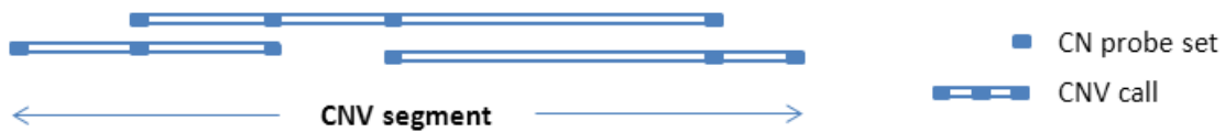
Figure 6.5: Schematic representation of a CNV segment defined by three overlapping CNV calls from two replicate data sets for the same individual.
