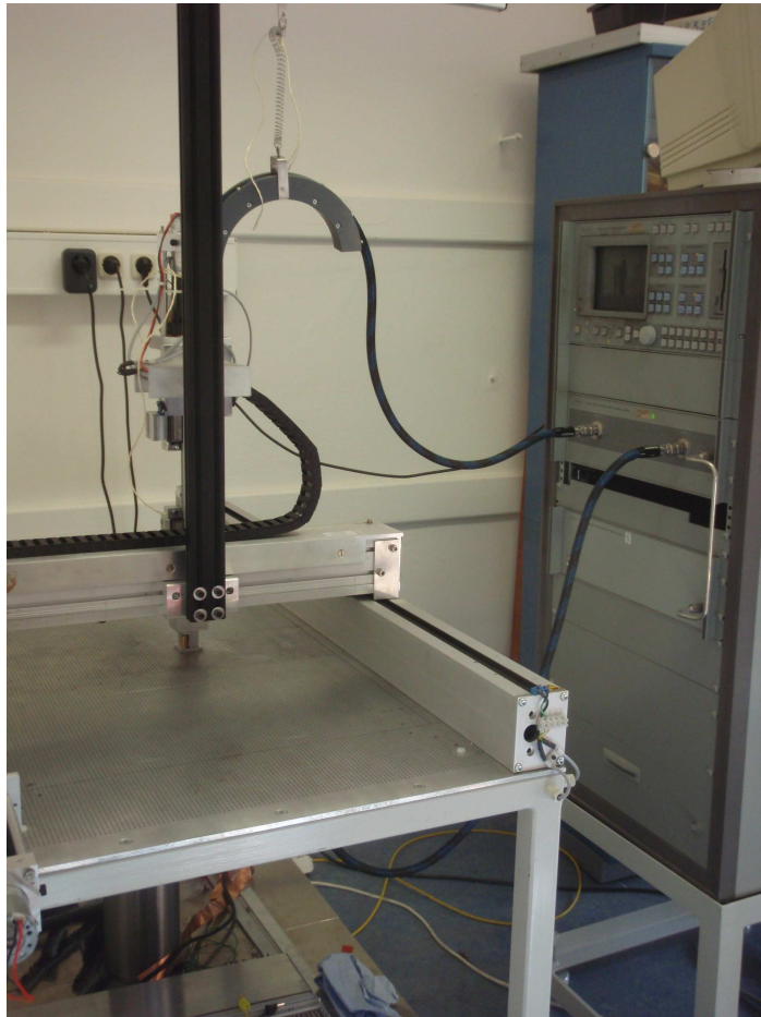
Figure 9: Photo of measuring table and vector network analyzer with two cables to the fixed and movable antennas
