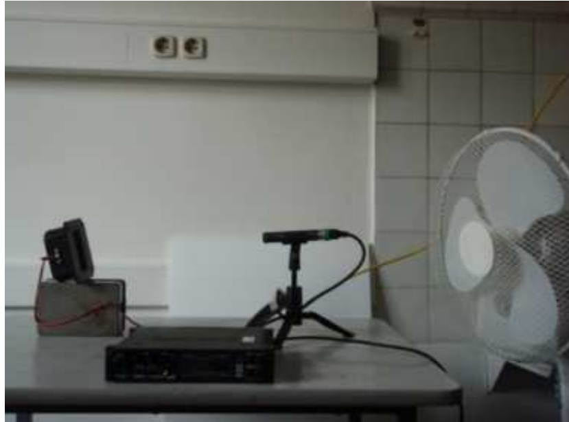
Figure 36: Setup with microphone (middle), loudspeaker (left), fan (right) and external sound card (middle in the front) in the “along”-configuration
