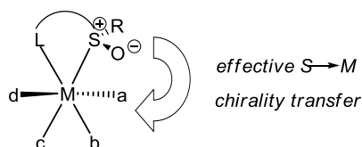
Figure 4. Facile chiral information transfer from a coordinated chelating sulfoxide to the neighboring octahedral metal center.
