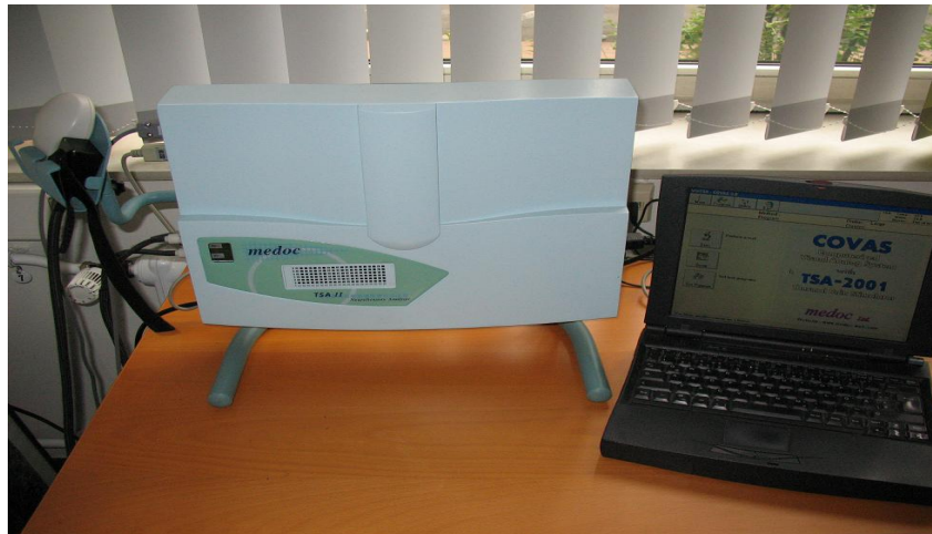
Abb.: 4.1 Thermal Sensor Analyser (TSA) von Medoc Advanced Medical Systems
