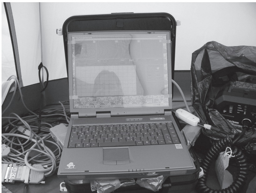
Figure 4-3: Heart Rate Recording Equipment II. Information collected in the artificial eggs was fed into the computer via a data logger. The software programme TTI VIPS enabled the observer to continuously monitor the quality of recordings. On the right hand side, the battery needed to power the artificial eggs is seen within its 'protective garment'.
