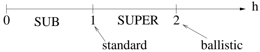
Figure 2.4: The exponent of the time dependent mean squared displacement controls two types of anomalous diffusion. For h = 1 we get normal diffusion. In the range 0 < h < 1 it is sub-diffusion, in the range 1 < h < 2 super-diffusion. Bigger values h \geq 2 are not in the realm of diffusion anymore.
