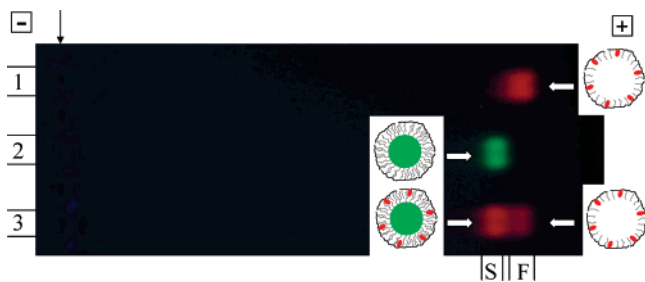
Figure 2. Quantum dots were coated with an amphiphilic polymer without (2) and with (3) incorporated ATTO590 dye. As control, empty polymer micelles with incorporated dye (1) are used. The three samples were loaded on a 1% agarose gel (arrow), and a voltage of 100 V was applied for around 1 h. During this time the negatively charged particles migrated toward the plus pole. Fast (F) and slow (S) migrating bands were observed by illumination the gel with a hand-held UV lamp. The empty polymer micelles (lane 1) can be seen as “fast” band by the red fluorescence of the ATTO dye incorporated in the polymer. The polymer coated quantum dots (without dye in the polymer, lane 2) can be seen as “slow” band by the green fluorescence of the quantum dots. Presumably, the polymer-coating procedure also produces empty micelles, which are not fluorescent and are not detected in our assay. The sample with the polymer coated quantum dots with dye incorporated in the polymer (lane 3) yields one “slow” band with orange fluorescent and one “fast” band with red fluorescence. The fast band (which migrated at the same speed as the control sample (1) with the empty polymer micelles) can be attributed to empty polymer micelles, which had been formed during the polymer coating process, and they can be observed due to the fluorescence of the ATTO dye incorporated in the polymer. The slow band (which migrated at the same speed as the polymer-coated quantum dots (2)) can be attributed to polymer coated quantum dots with dye incorporated in the polymer. The emission from these nanoparticles appears orange, as part of the energy absorbed by the quantum dots is transferred via FRET to the dye in the polymer, and for this reason an overlap of the quantum dot and dye fluorescence is observed.
