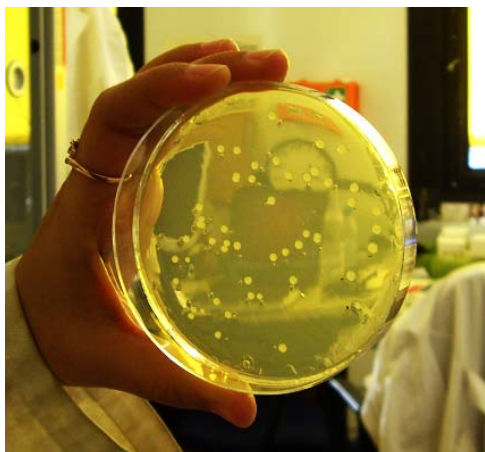
Fig 3.4.23. Bacterial E.coli . grows with contact with P(MDO-MMA-DMAEMA)•BrC 12 H 25 containing 40 mol% of MDO and 20 mol% of ion.
