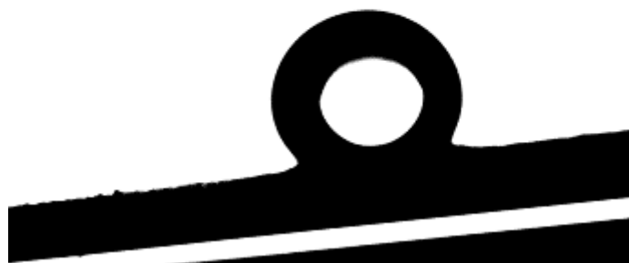
Fig 3.3.10. Contact angle of the fiber mat (polymer with 10 mol% of BMDO, 88 mol% of ion, quaternary reagent: \text{BrC}_{12}\text{H}_{25} ) by electrospinning.
