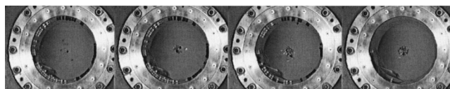
FIG. 4. Macroscopic nucleus formation from beads (5 mm). The conditions are similar to those in Fig. 3. The object at magnet center is a U.S. dollar bill, which is paramagnetic and is attracted to the bore tube wall.
