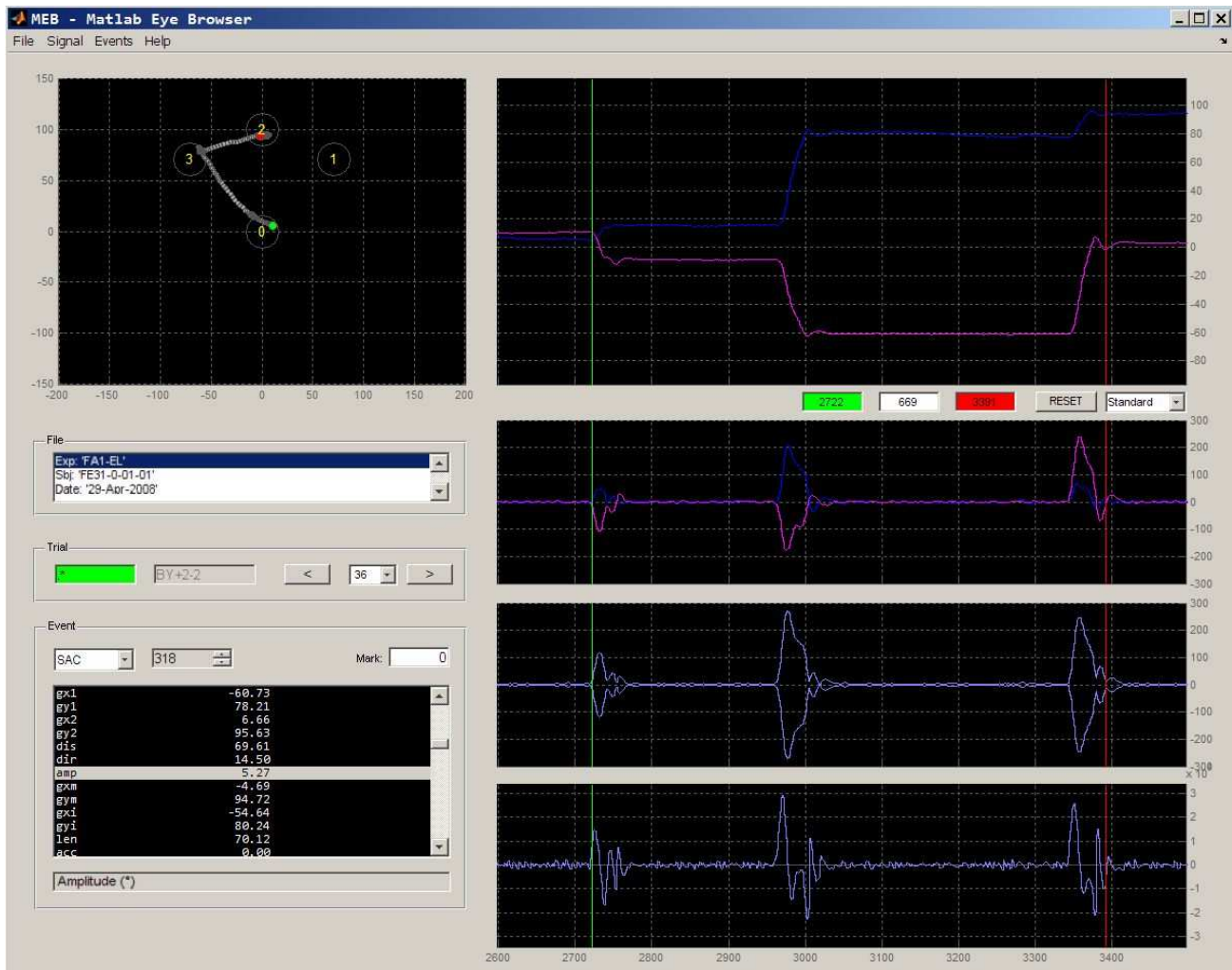
Figure 1. Main screen of the Matlab Eye Browser (MEB). Time plots on the right are selected to show gaze position, gaze velocity, component velocity and gaze acceleration respectively. Vertical start (green) and end (red) marks enclose a sequence of three saccades.
